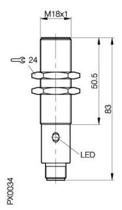
Inductive Sensors BES 516-539-S 4-H M18x1 x 83 normally-closed Sn=5mm shielded
